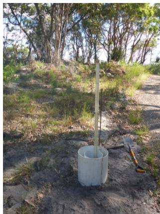
Photograph 13 Double ring infiltrometer apparatus set up at location INF1.
