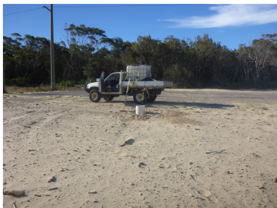
Photograph 15 Double ring infiltrometer apparatus set up at location INF3.
