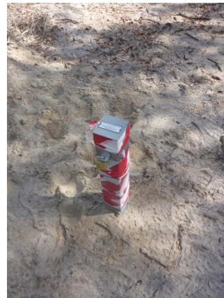
Photograph 12 Installed Piezometer PZ1 at the location of BH7.
