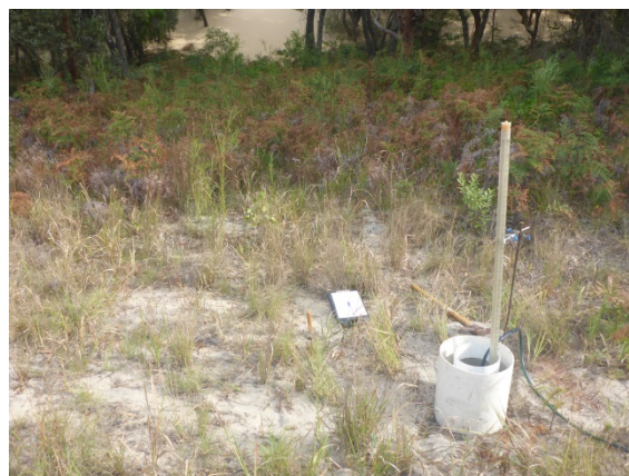
Photograph 16 Double ring infiltrometer apparatus set up at location INF4.
